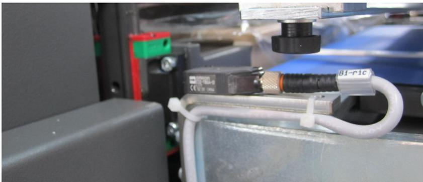
Top adjustment is for sensitivity minimum and maximum
