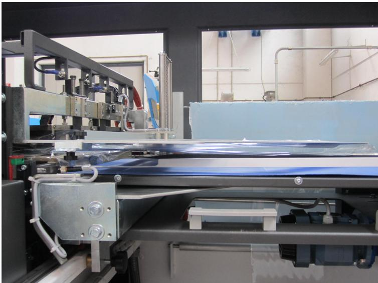
Belts are adjustable from both sides by loosening nut and turning hex bolt clockwise to tighten belt and counter clockwise to loosen belt.
