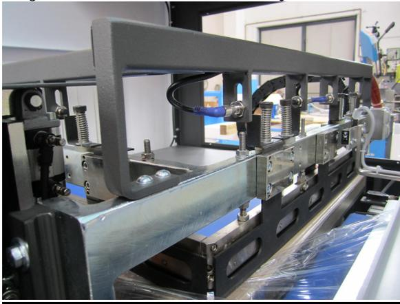
Safety sensor should be set 1/8" above metal bracket. Sensor gap should be set 3-4mm from bracket
