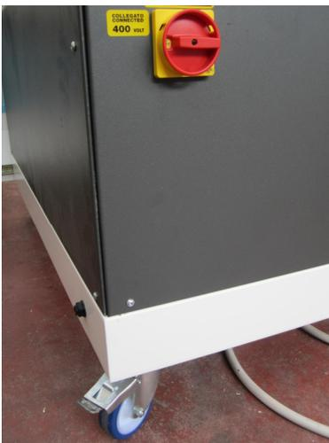
Machine has threaded casters that can be adjusted
