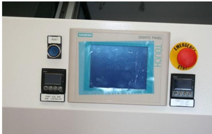
1. **Start switch**- Starts the machine for automatic production. The push button is illuminated when depressed enables the machine to operate in manual mode.
