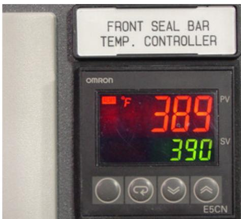
You may increase the temperature by pressing the up arrows key or decrease by pressing the down arrow key. The two buttons to the right are for programming functions only – Do Not Touch!
