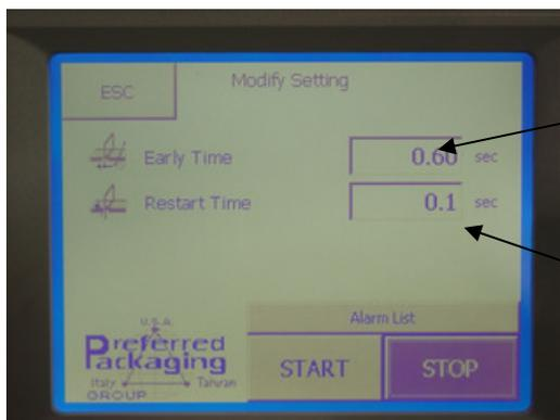
**Early Time** -If set on zero, package must clear seal bar area and photo eye before seal bar activates. Higher number seal bar will activate prior to package clearing seal bar.
