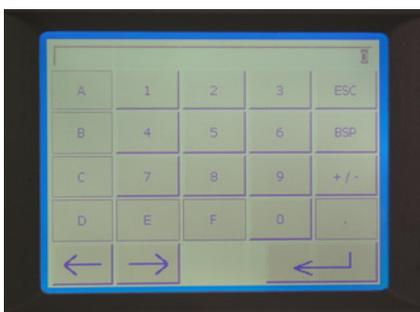
**Access screen for selecting program memory and used for selecting numerical setting on machine**
