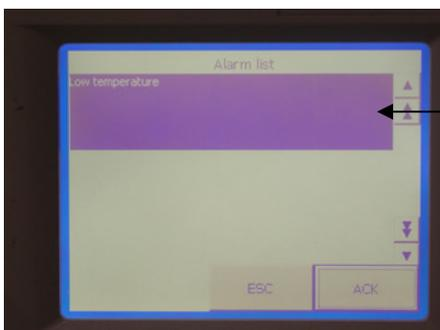
Low temperature on sealing bars will not allow the machine to operate
