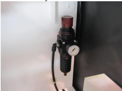
7. Make sure your air supply is connected and you have a minimum 80 psi. /6 Bar
