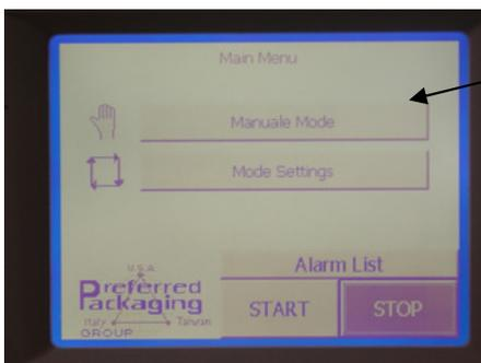
Manual mode=Allows operator to make manual adjustments to machine.
